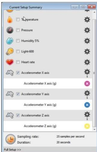
6. Click Full Setup, to program the data logger's sample rate, number of samples, units of measurement, and other options
