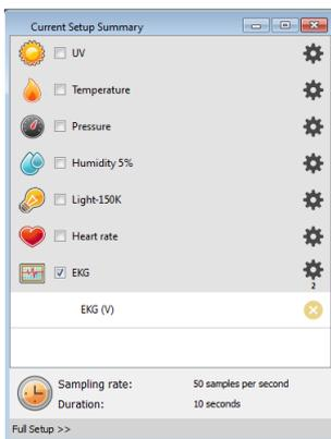
5. Click Full Setup, located at the bottom of the Current Setup Summary window to program the data logger's sample rate, number of samples, units of measurement, calibration and other options
