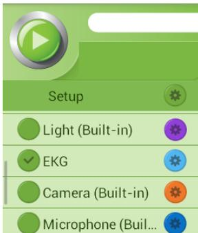
5. Make sure the icon next to the sensor is checked (
