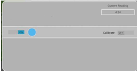
2. Flip the Calibrate switch to On
