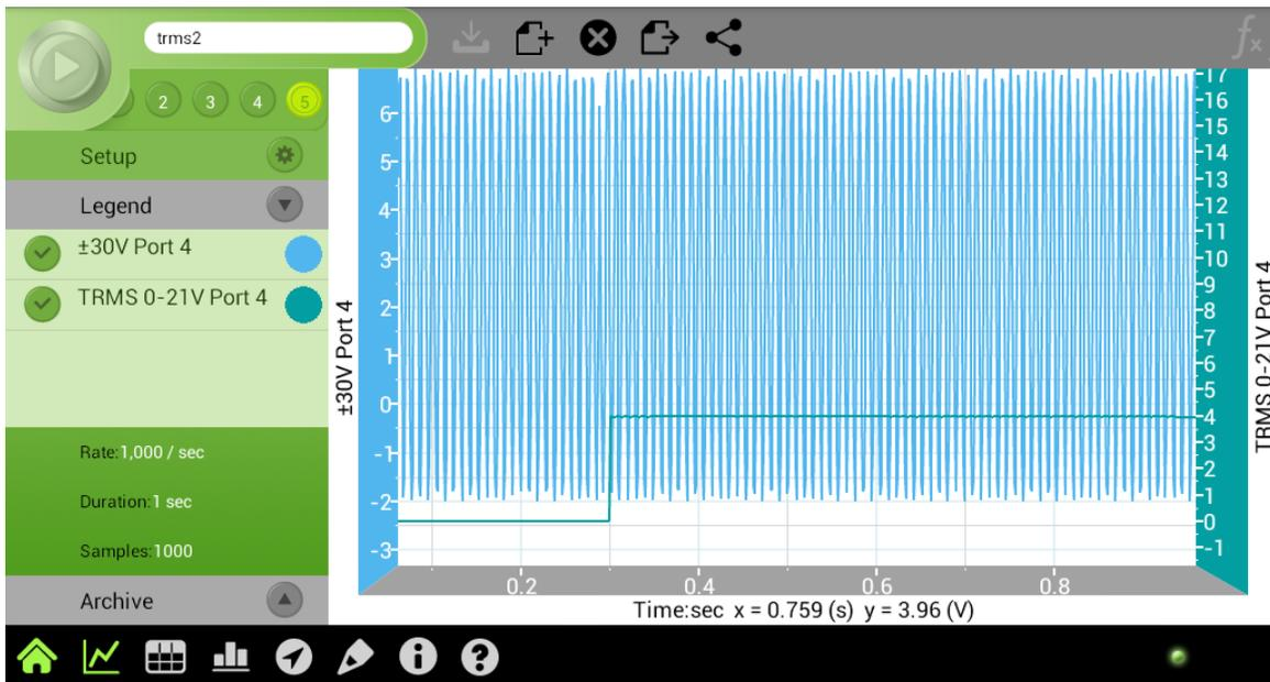
Typical graph of this experiment in MiLAB Mobile. Blue represents the Voltage reading, green the TRMS reading.
