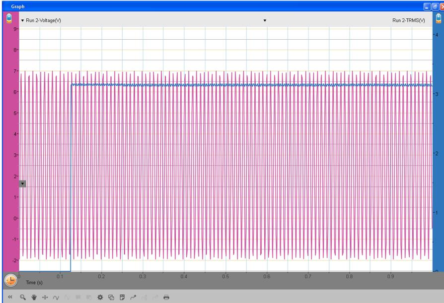
Typical graph of this experiment in MiLAB™ for Desktops. Red represents the Voltage reading, blue the TRMS reading.
