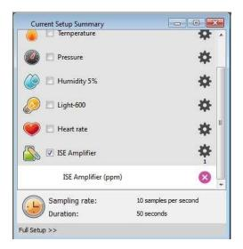
6. Click **Full Setup**, located at the bottom of the **Current Setup Summary** window to set which ISE electrode you are using and to program the data logger's sample rate, number of samples, units of measurement, and other options
