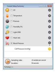
Click Full Setup, located at the bottom of the Current Setup Summary window to program the data logger's sample rate, number of samples, units of measurement, and other options
