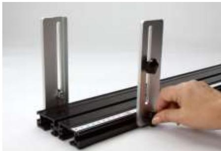
2. Mount the Photogate or Distance sensor on the bracket using the star-knobbed bolt provided.
